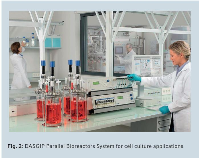
Fig. 2: DASGIP Parallel Bioreactors System for cell culture applications
