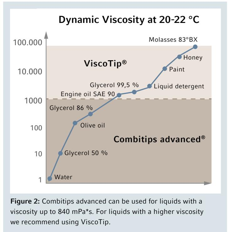
**Figure 2:** Combitips advanced can be used for liquids with a viscosity up to 840 mPa\*s. For liquids with a higher viscosity we recommend using ViscoTip.
