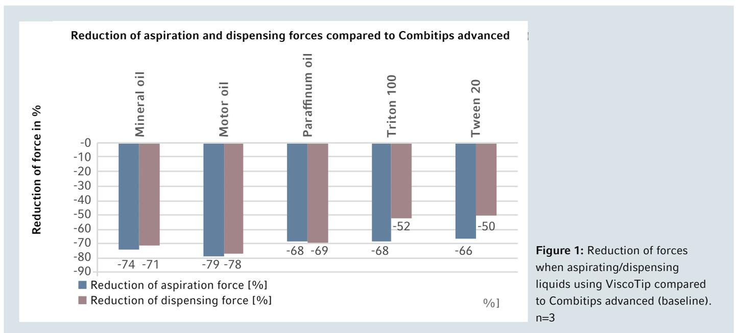
**Figure 1:** Reduction of forces when aspirating/dispensing liquids using ViscoTip compared to Combitips advanced (baseline). n=3
